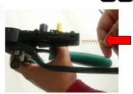
Insert the strip of contacts into the feed unit. Kontaktstreifen in Vorschubeinheit legen.
