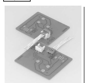
1.25 mm pitch crimp type connector. This connector system has excellent operational advantages due to its top entry style. In addition, with the wires on the side, it is low profile, similar to a side entry style.
