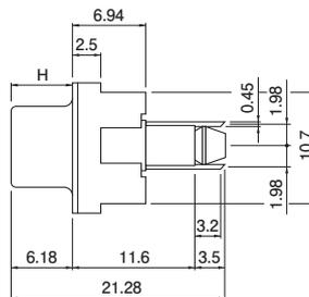
H: Height of the lock screw block (for Types A & B)
