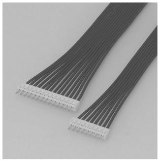
A dimension of 2.0mm pitch, 4.0mm mounting height and 2.9mm depth. This board-in type connector will enhance the mounting density of the PC board even further as well as improve rationalization and reduce the total cost of production. This product will be suitable for the internal connector of low profile equipment, such as audio equipment (including car audio) and the STB.
