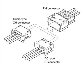
This is a space-saving 1.5 mm pitch wire-towire connector that mates with both crimp and IDC type sockets.
