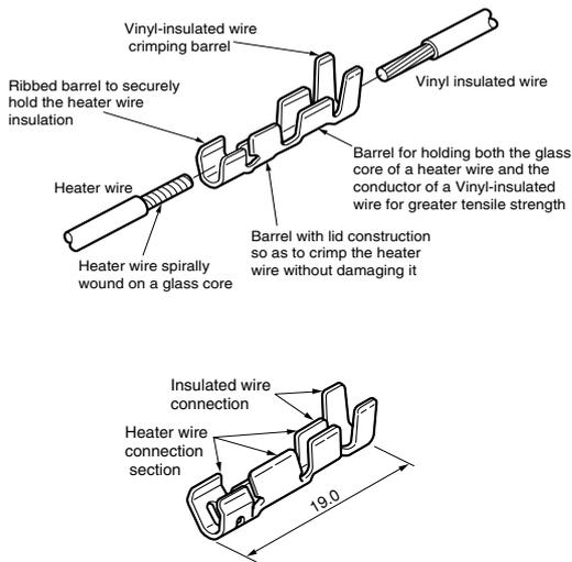
***This splice is used to connect a vinyl-insulated wire to a defrosting heater wire of a refrigerator or a freezer.***
