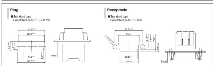
Note: 1. Punch holes in the panel according to the figures shown above. Burrs must be removed.
