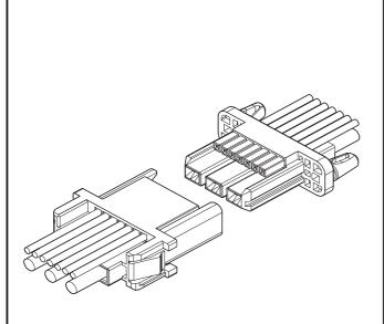
This connector is a hybrid type double-row drawer connector with combined signal and power supply circuits to connect the units. In the signal part, the number of parts reduced by connecting the crimping contact directly.
