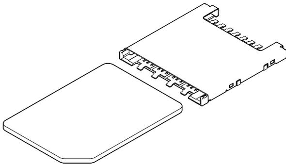
**A manual insertion type connector for SIM card and Mini B-CAS card used in mobile phone**
