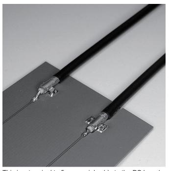
This is a terminal to fix a coaxial cable to the PC board. By press-fitting the dimple on the terminal foot portion into the PC board, the terminal is fixed when installing it onto the PC board and the soldering work is improved.
